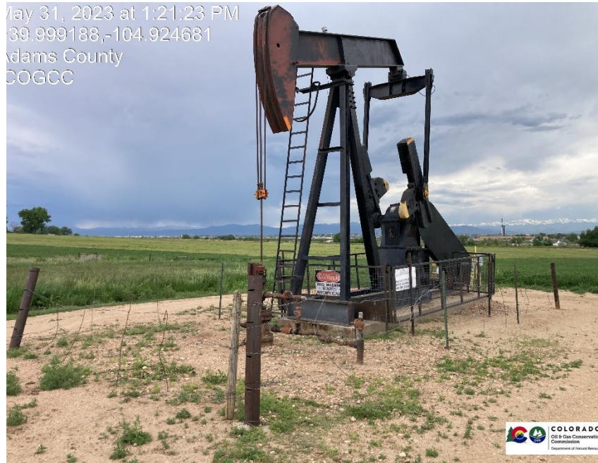
Pic 1 wellhead / pump jack
