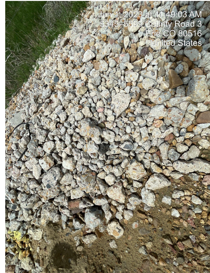
Photo 10. Photo of crushed concrete on fill slope.
