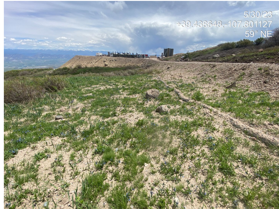
Photo 22. Photos show offsite deposition of sediment and road base gravel downslope of the access road. Wattles have been overtopped (right).
