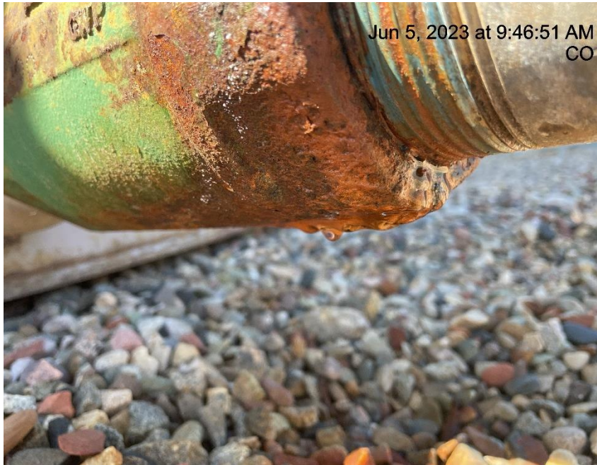
Photo # 9438 Valve on production tank leaking fluid
