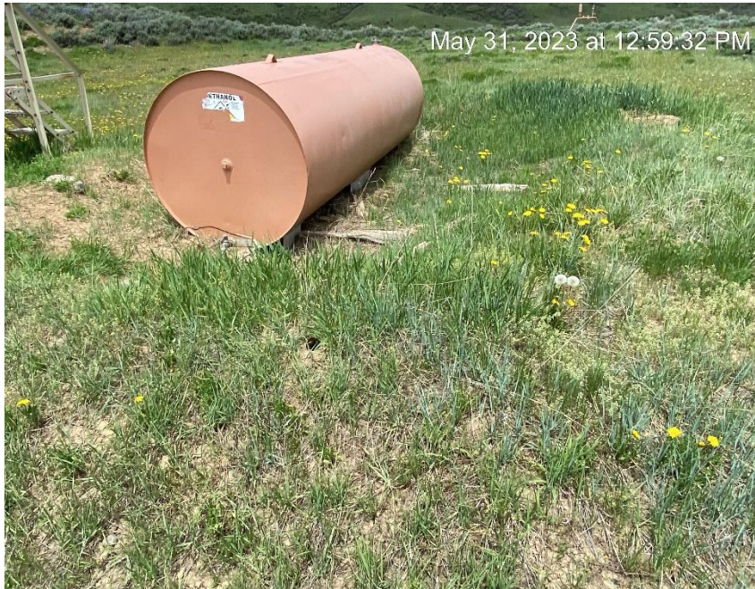
Missing labels. Insufficient containment.
