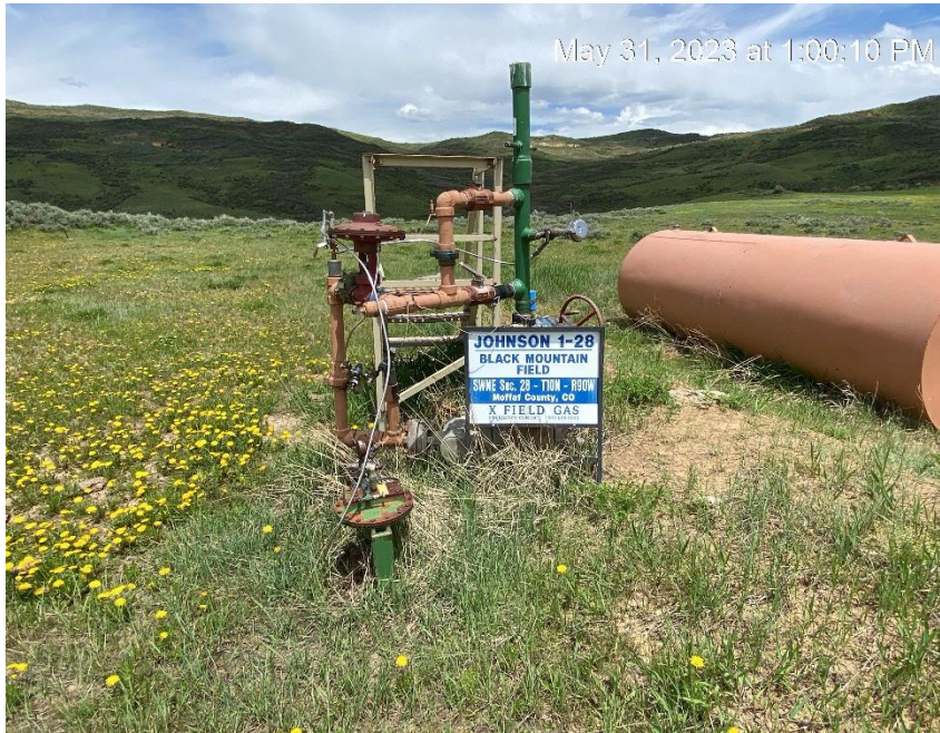
Chemical pump and methanol tank without adequate containment
