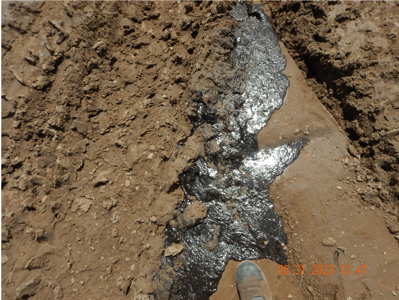
Photo 5. Photo taken from the southwestern well pad. Photo illustrates oily waste which has not been cleaned up and disposed of properly. The extent was unclear due to vehicle traffic but it appears to have mixed with stormwater. Note- there were pieces of rig liner throughout the western well pad that has been disturbed.
