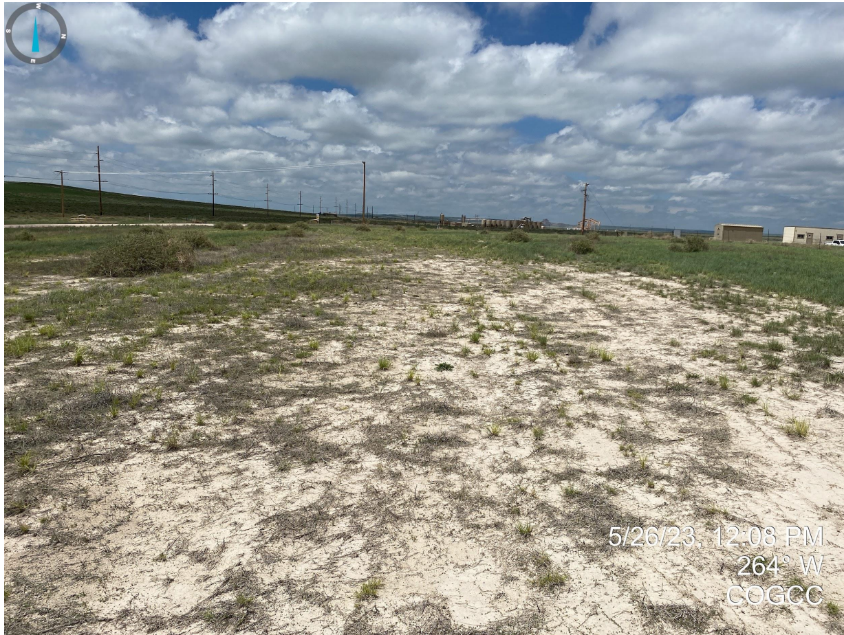
Photo 3. Southern interim area. The interim areas are not progressing towards reclamation standards with evidence of non-uniform vegetation cover resulting in areas of bare soil and undesirable vegetation (e.g. kochia) was observed growing throughout. Additional reclamation activities are required in order to meet Rule 1003 standards.
