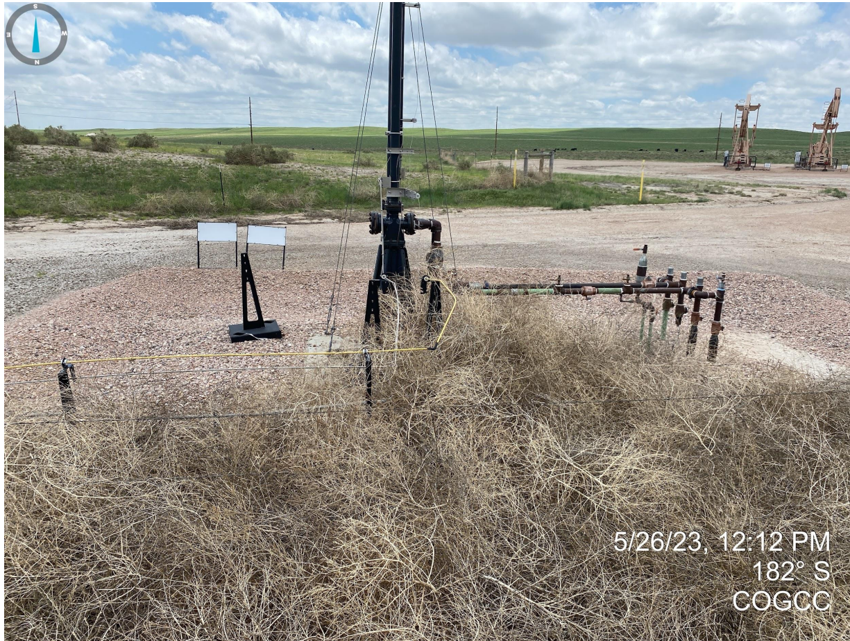
Photo 7. Tumbleweed accumulations around flare unit will need to be removed as they present a fire hazard.
