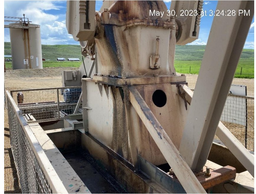
Equipment leak and staining
