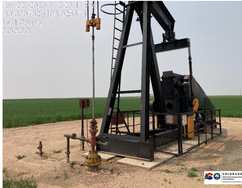
Pic 1 wellhead / pump jack
