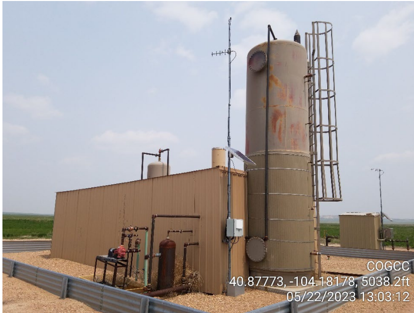
Photo 5 – Heater Treater
