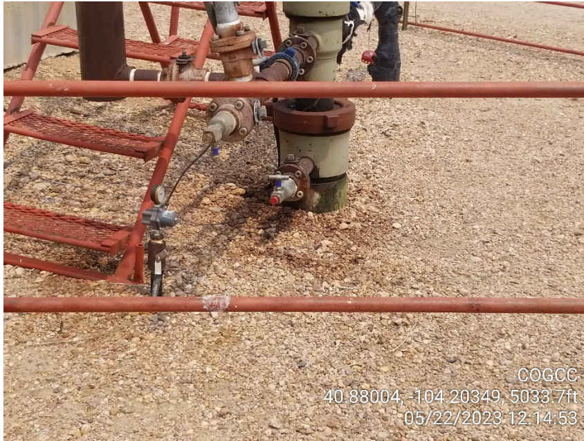
Photo 7 – Stained Soil at Wellhead
