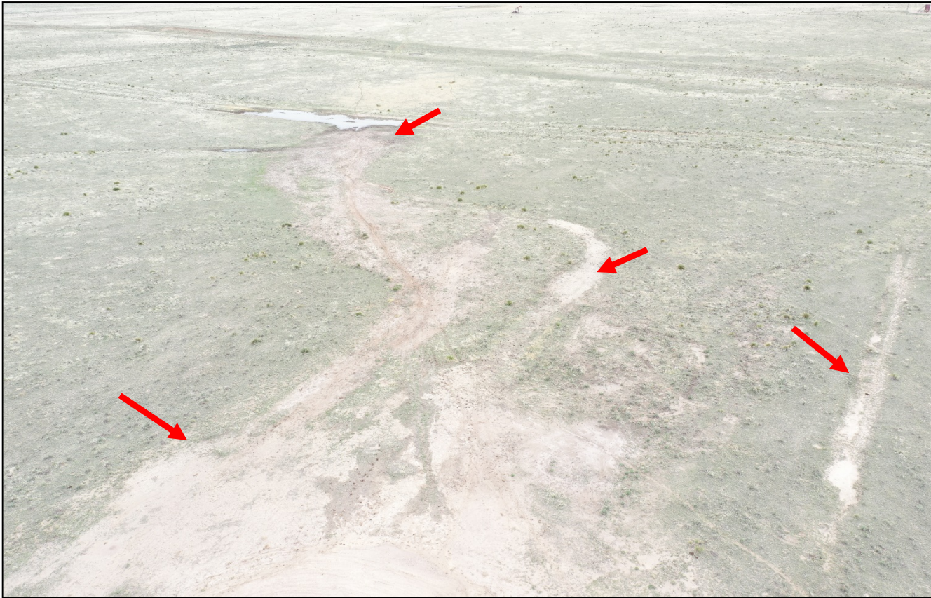
Photo 2. Drone aerial photo facing northwest from the Foster #1 wellsite. There is multiple impacted areas from previous spill. Site investigation and remediation will need to occur.
