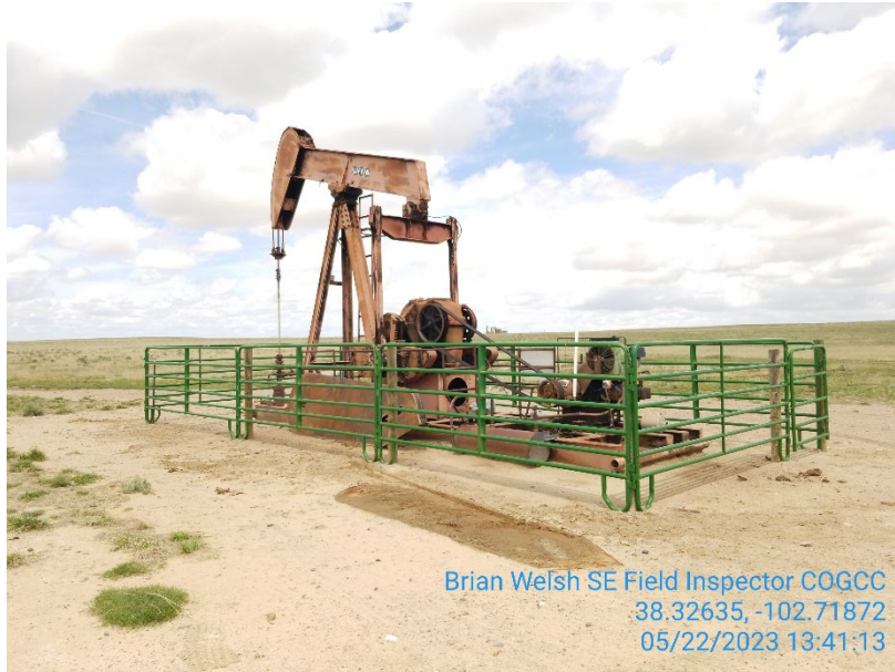
1. Belt guard at pumping unit has been moved to inside fenced area
