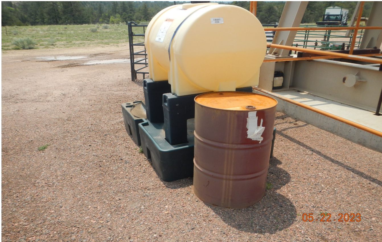
Photo 3. There is an unknown barrel with no labeling or containment.
