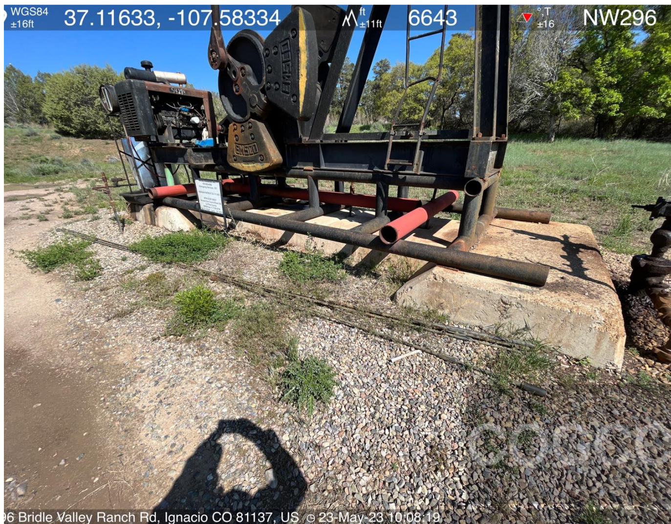
Photo #5. View of stored sucker rod on ground.
