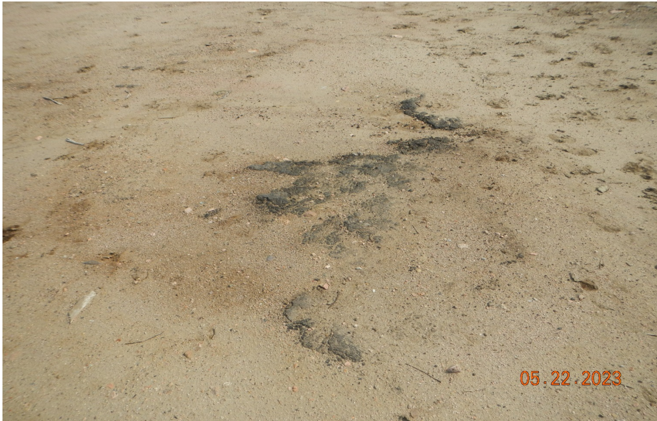
Photo 5. There is oil stained soils at center of location that needs to be cleaned up.
