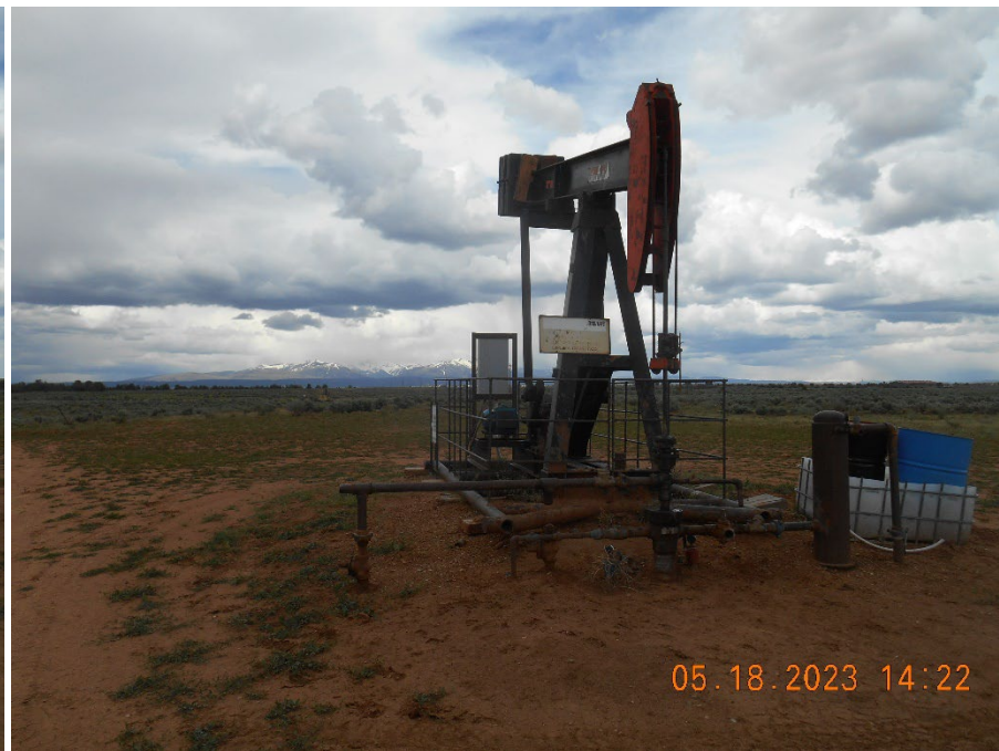
Wellhead with pump jack.
