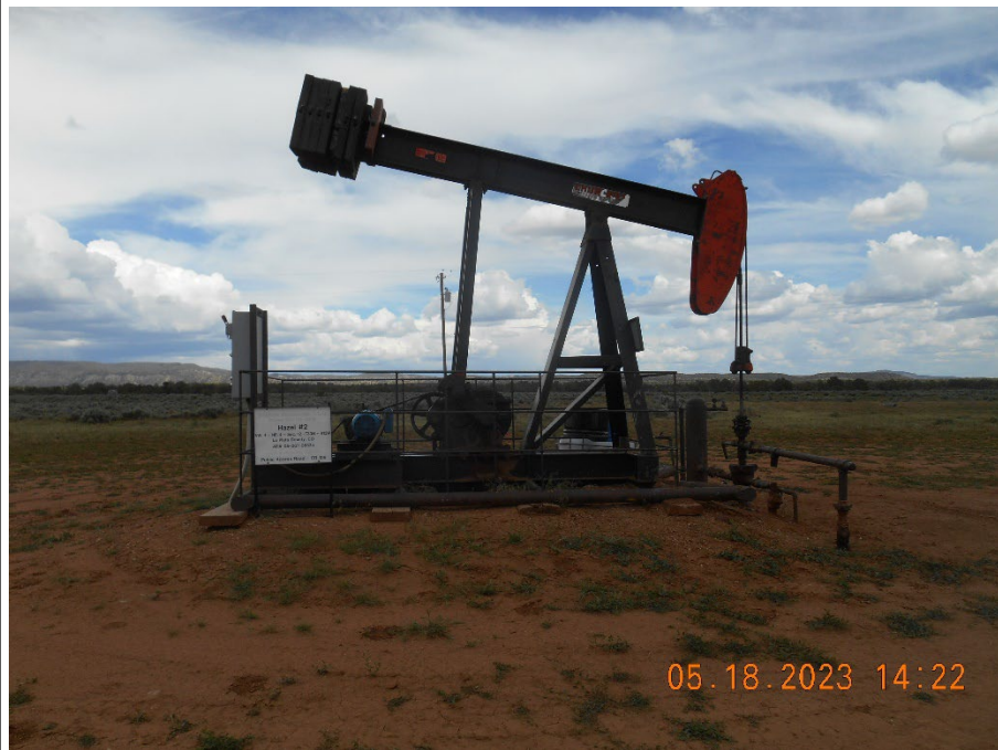
Wellhead with pump jack.
