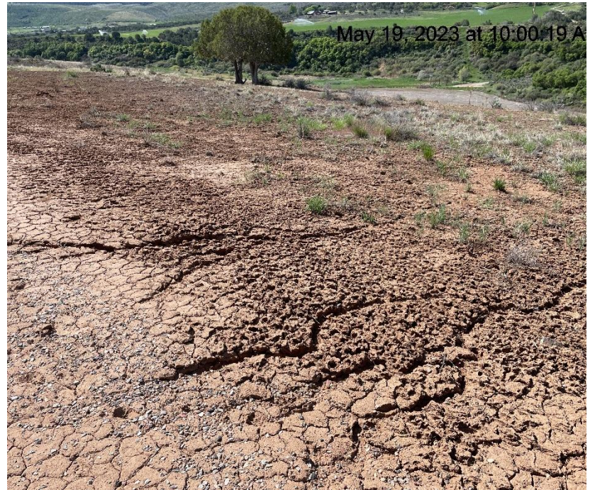
Photo # 8235 Erosion & transport of sediment off location into vegetation/insufficient BMP's (South side of location)
