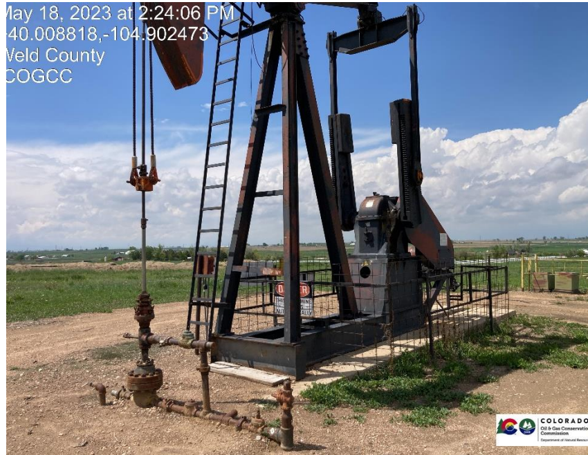
Pic 1 wellhead / pump jack
