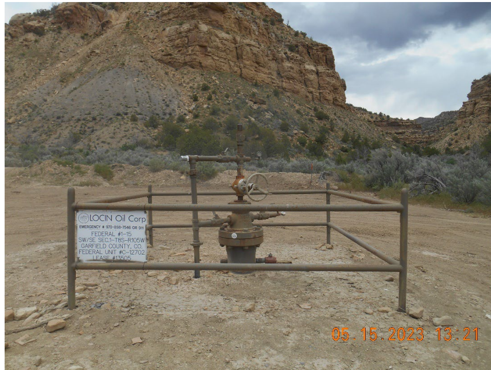
Wellhead with fence and sign
