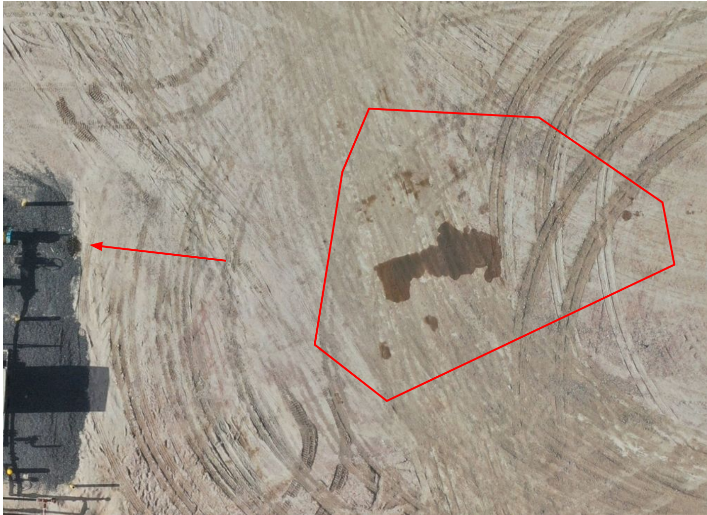
Photo 2. Drone aerial imagery illustrates a spill (red circle and red arrow) located along the southwestern well pad.
