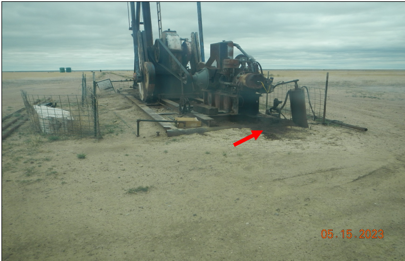
Photo 8. The fence is not up at the backside of the pumpjack to prevent livestock entry. There is oil stained soils shown red arrow that need to be cleaned up.
