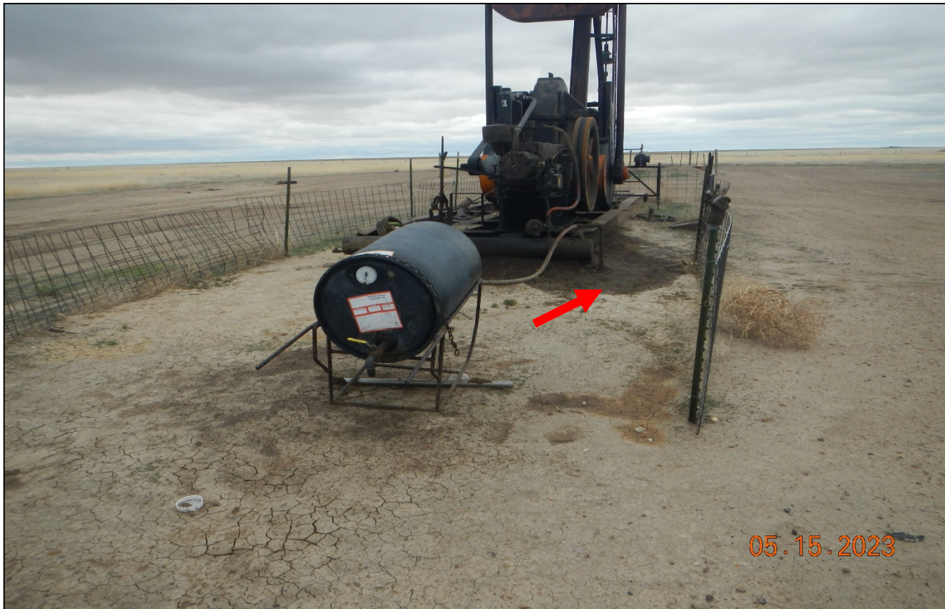
Photo 2. There are oil stained soils at the base of the pumpjack that need to be cleaned up. There is no secondary containment of the chemical barrel.
