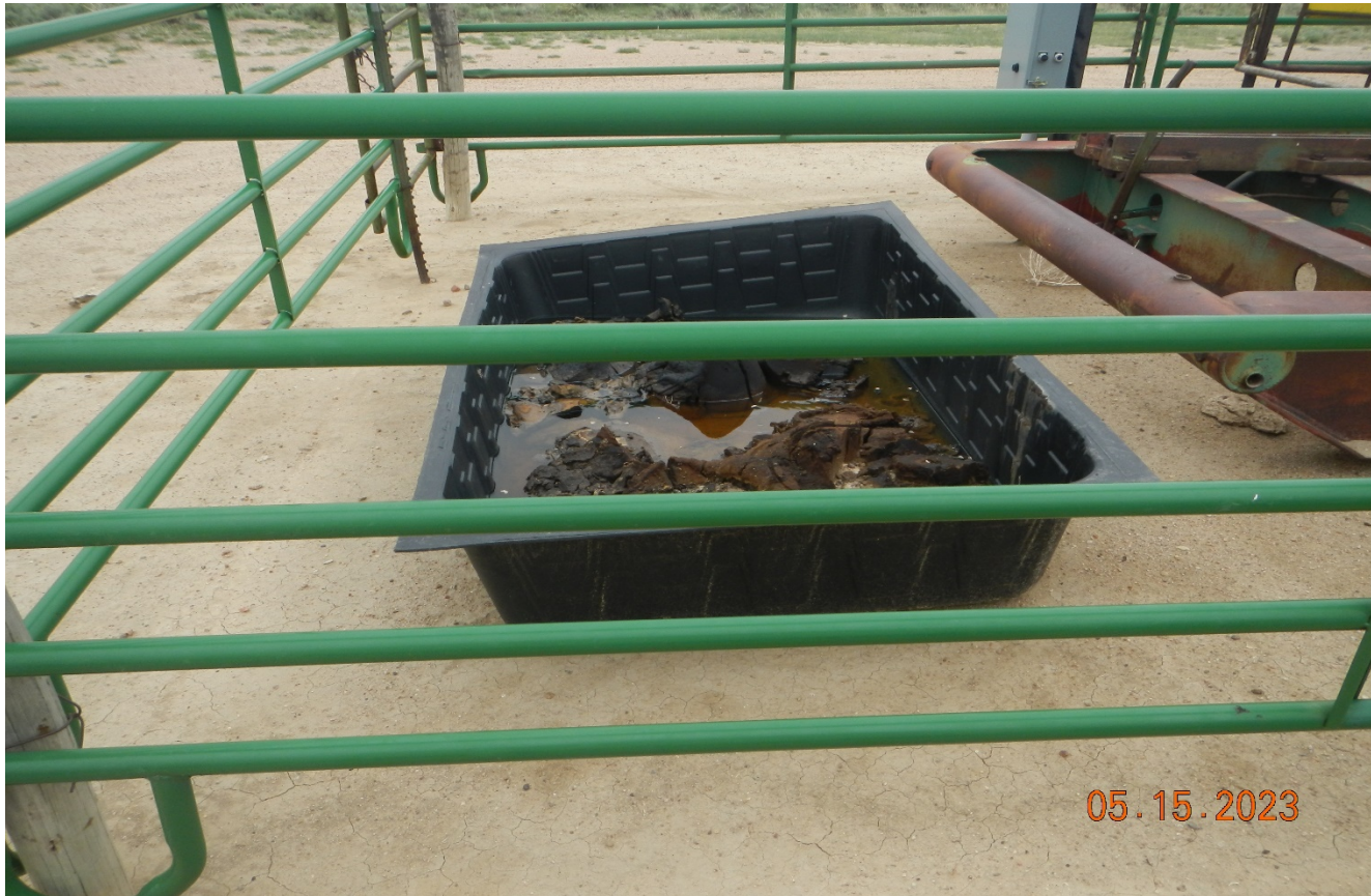
Photo 5. There is oily material being stored in this containment which needs to be removed and properly disposed.
