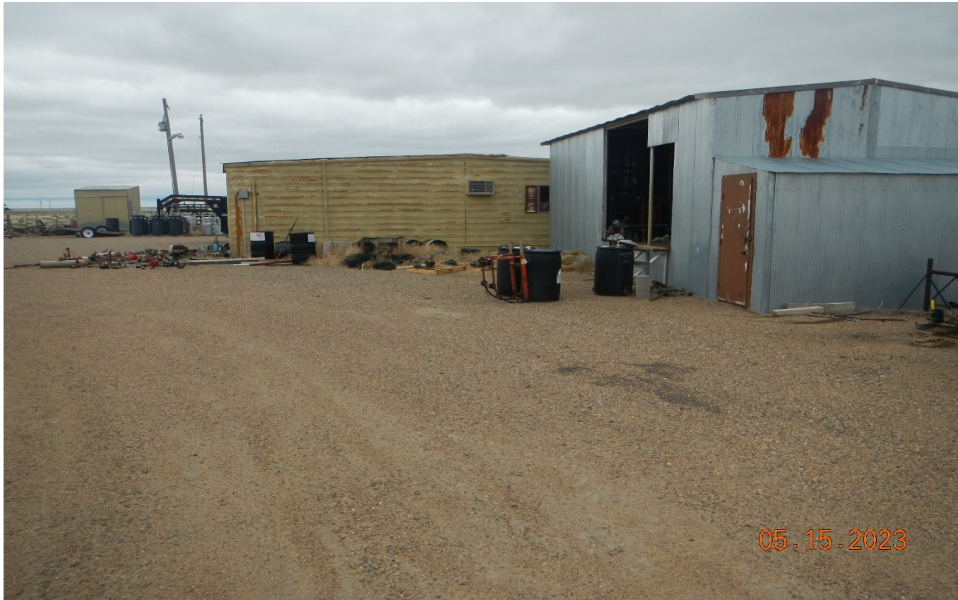
Photo 12. There are several chemical barrels on location with faded labeling and no secondary containment.
