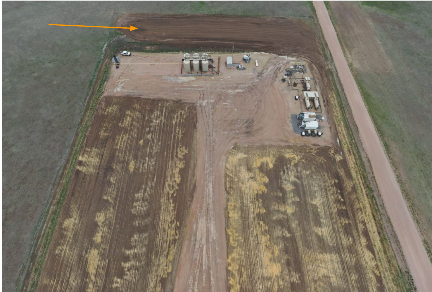
Photo 1. Drone aerial imagery illustrates the northern half of the location. Photo illustrates interim reclamation has been performed; however, interim reclamation is not complete due to the lack of soil stabilization on the topsoil stockpile (orange arrow) and throughout portions of the interim reclamation area.
