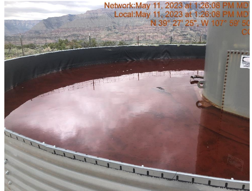
Photo #9939 Secondary containment capacity reduced
