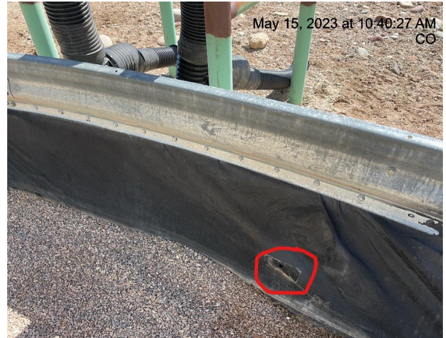
Photo # 7780 Containment liner needs maintenance
