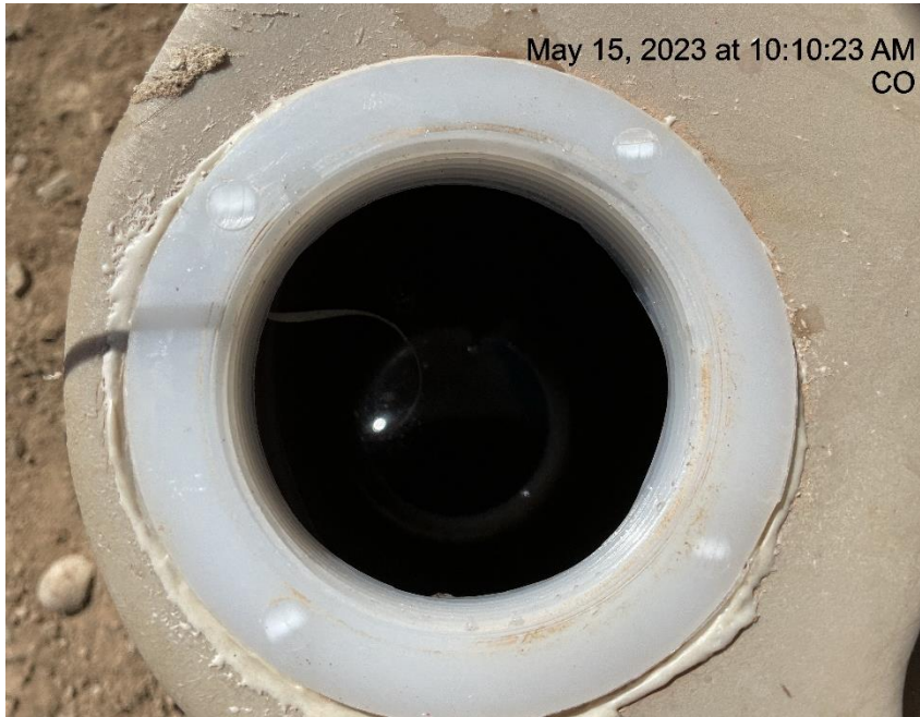
Photo # 7734 Chemical containment full/failure to maintain chemical BMP
