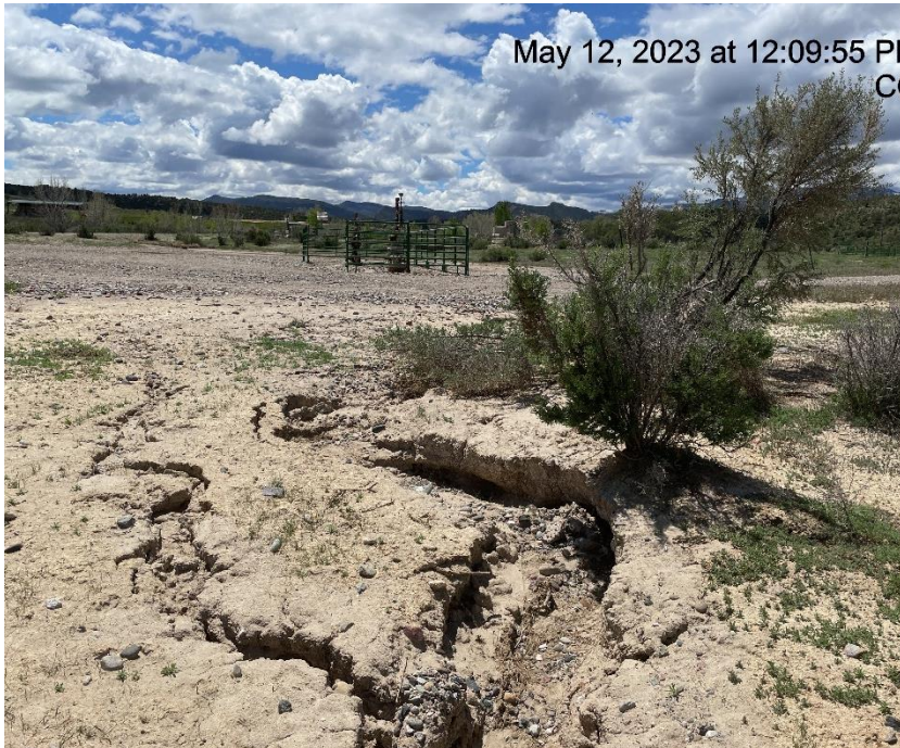
Photo # 7634 Erosion & transport of sediment/Insufficient run off controls/BMP's
