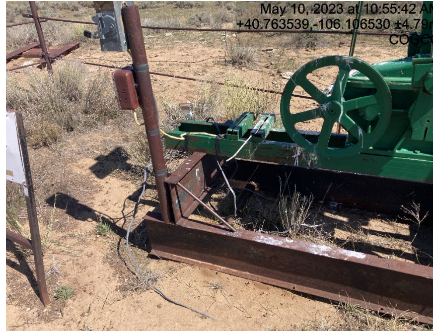
Pump jack not in service and wires are laying on the ground.
