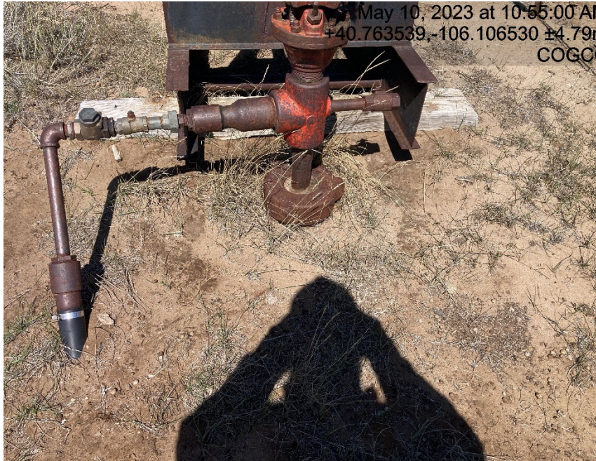
Lack of Braden head access
