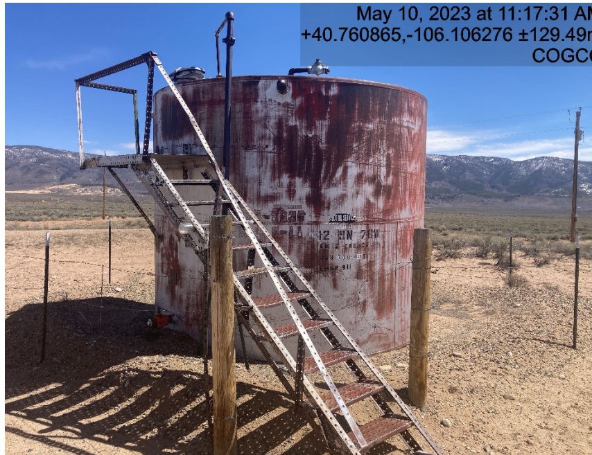
Tank battery lacking proper signage
