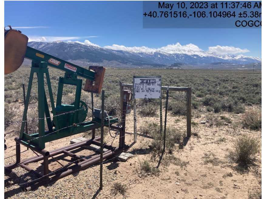
Well head sign is lacking information
