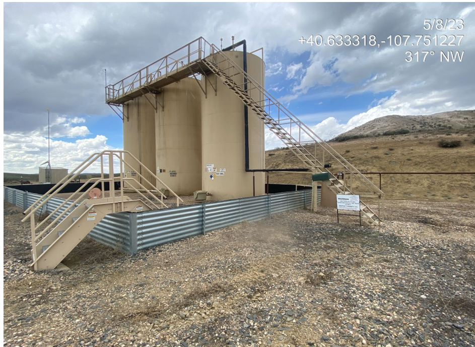
Photo 15. Photos show production areas. The battery sign does not comply with Rule 605.e (left). The wellhead sign does not comply with Rule 605.d (right).
