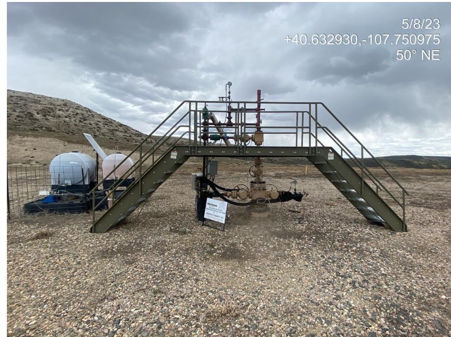
Photo 15. Photos show production areas. The battery sign does not comply with Rule 605.e (left). The wellhead sign does not comply with Rule 605.d (right).
