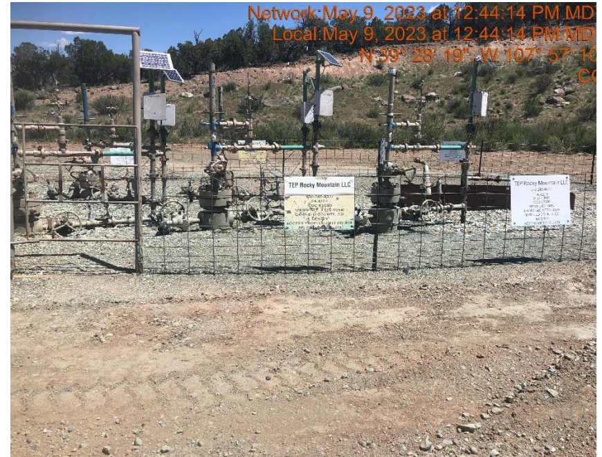
Photo #9901 Multiple wellhead signs weathered and not legible.
