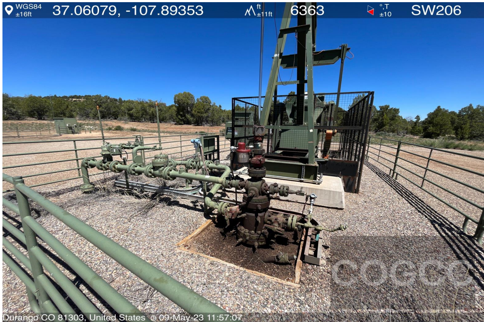
Photo #2. View of wellhead assembly.
