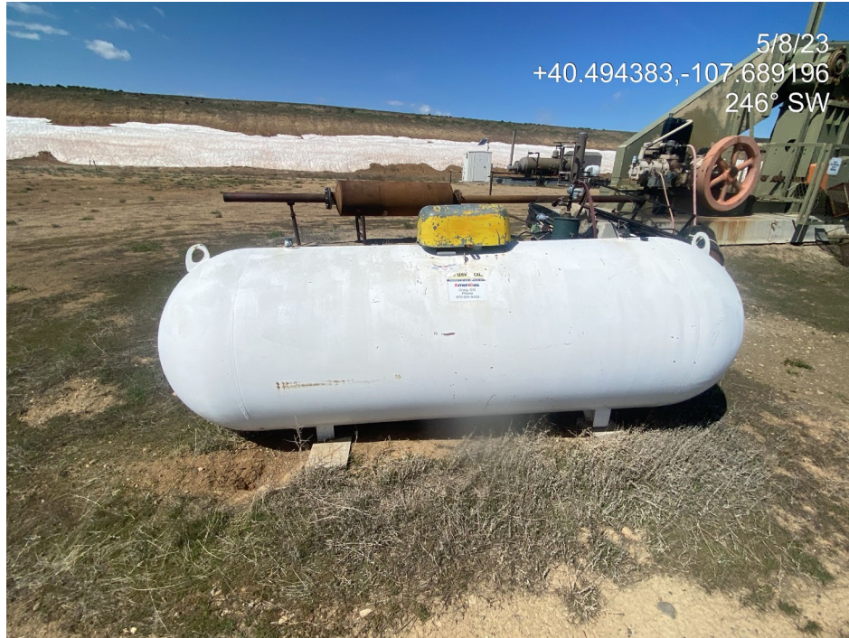
Photo 17. Photos show a tank at the pumpjack lacks safety labeling.
