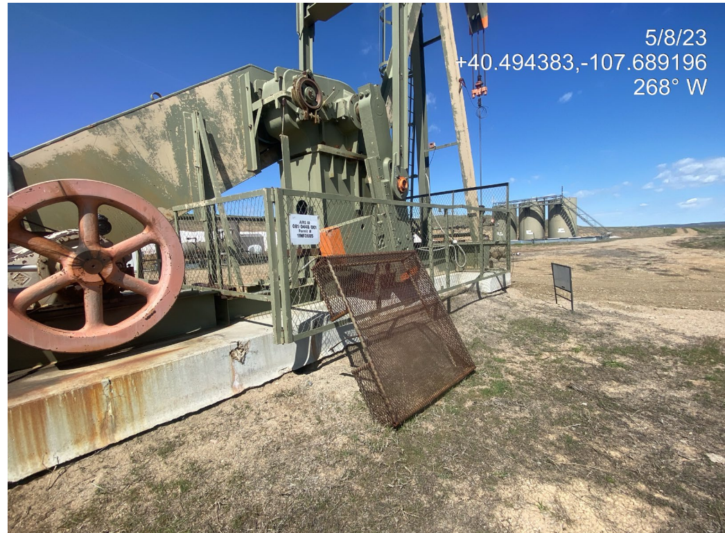
Photo 16. Photo shows the guard not installed on the pumpjack.
