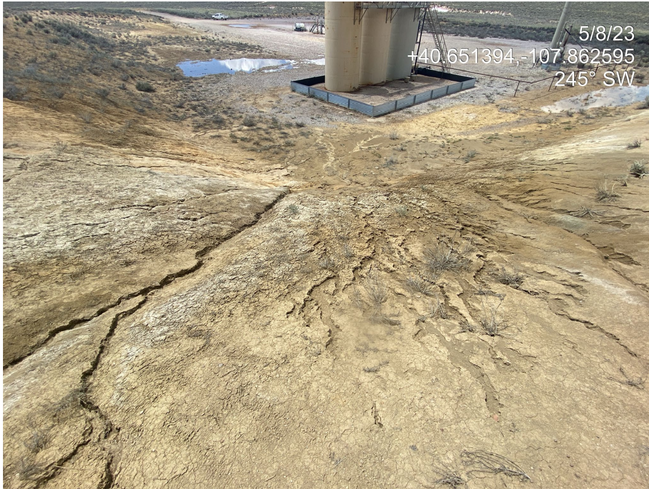
Photo 8. Photo shows rill erosion on the unstabilized cut slope to the northeast.
