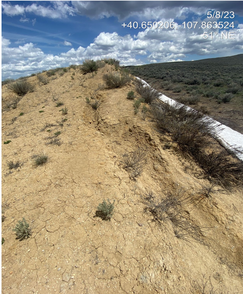
Photo 4. Photo taken from the south of the Location shows gully erosion occurring on unstabilized slopes.
