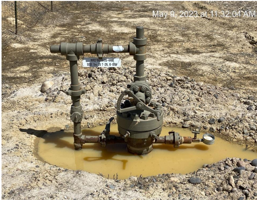
Inaccessible Bradenhead
