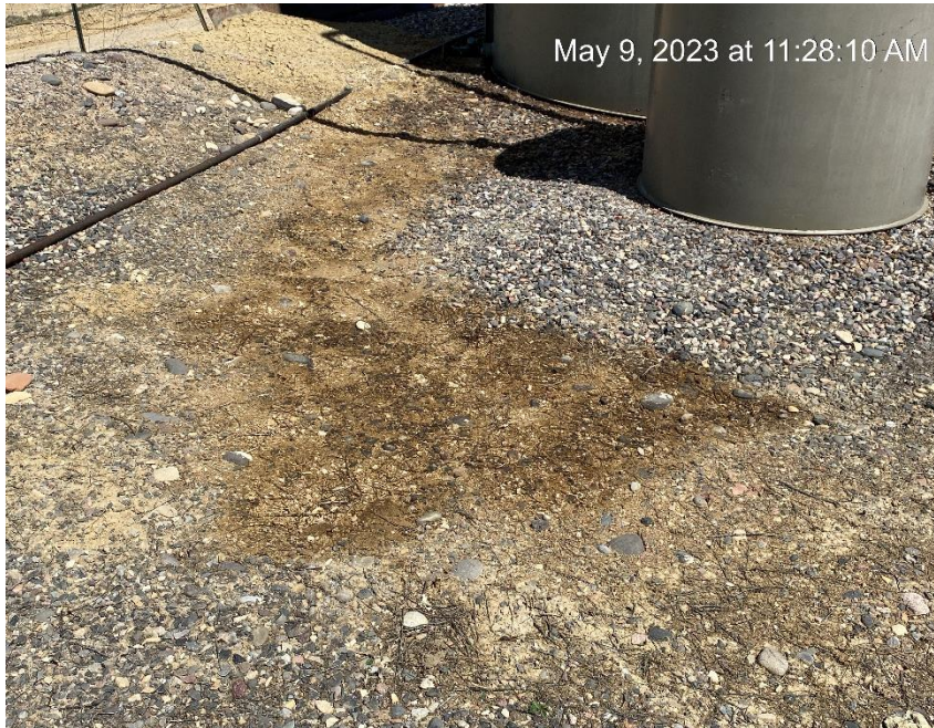
Soil staining inside tank battery containment
