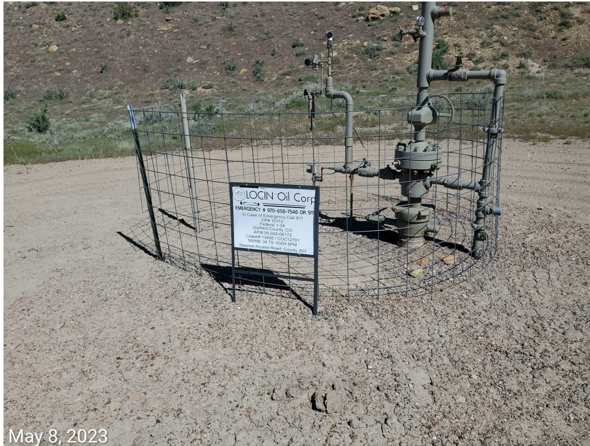
Photo 4: Wellhead. Tank has been removed.
