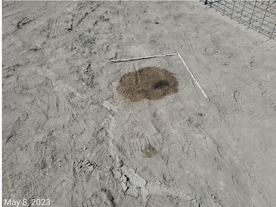
Photo 8: Stained soils on Location; stained soils require cleaning/remediating. 6 foot (3'x3') measuring stick used for reference.
