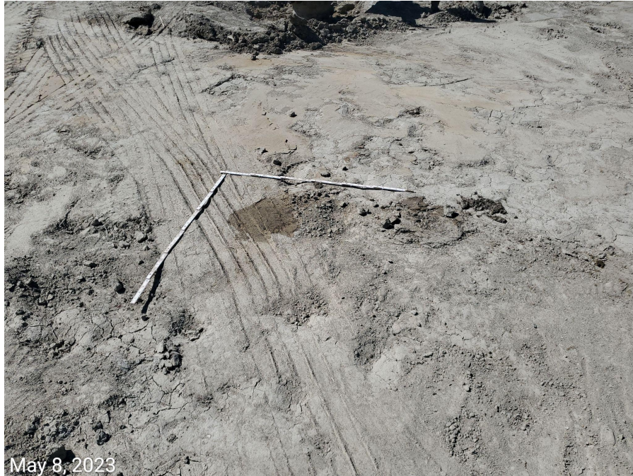
Photo 9: Stained soils on Location; stained soils require cleaning/remediating. 6 foot (3'x3') measuring stick used for reference.
