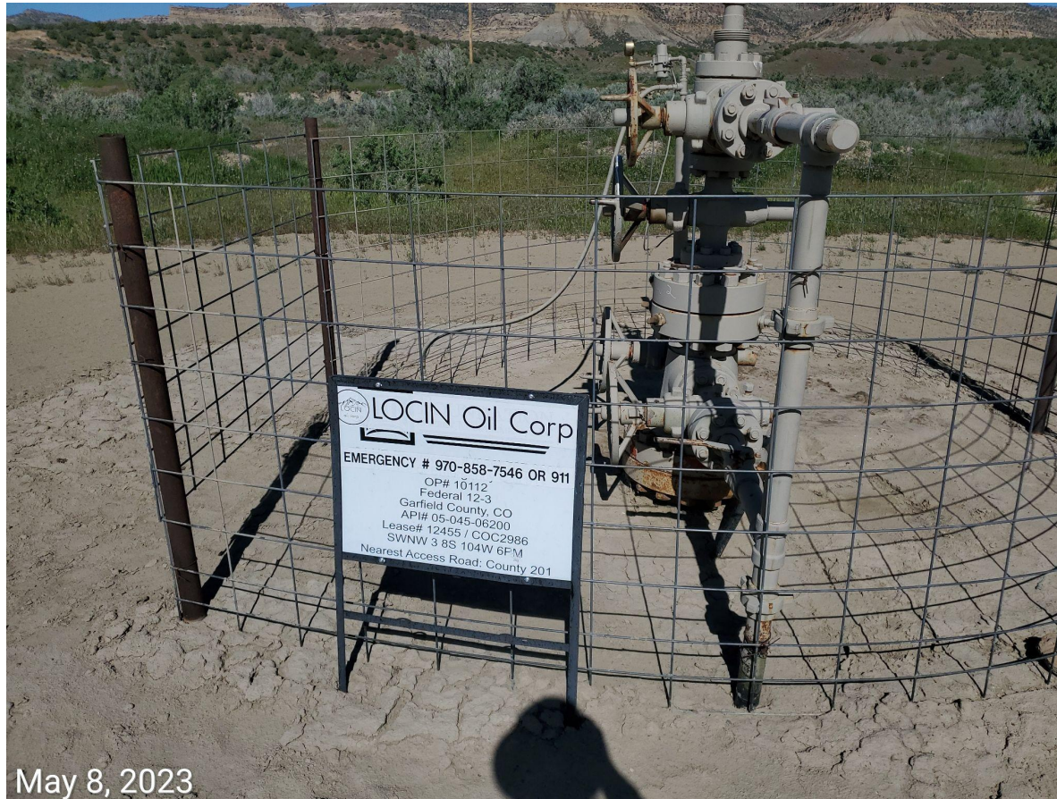
Photo 6: Wellhead. Methanol container removed.
