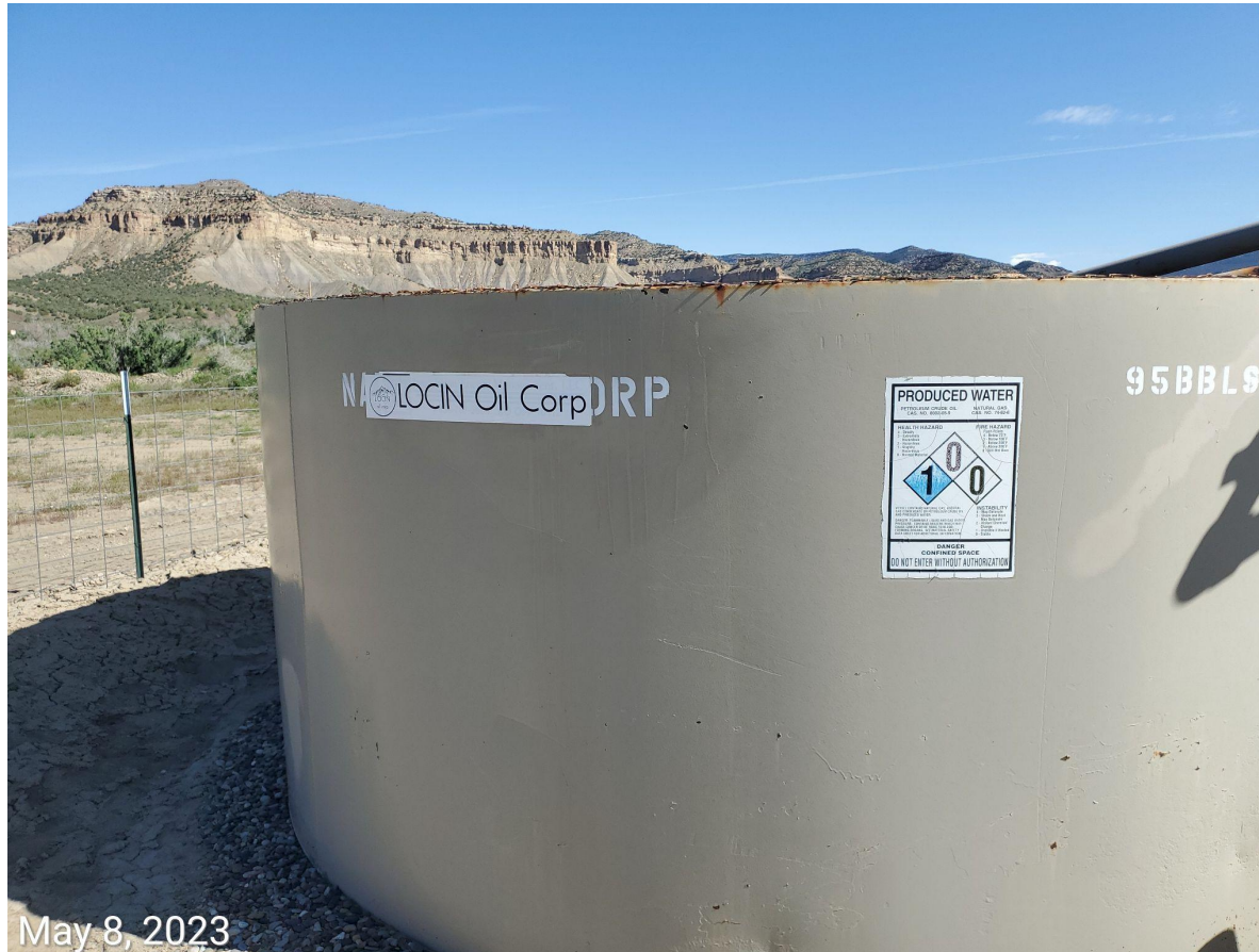
Photo 3: Signs/labels at tank do not comport with Rule 605.h.
