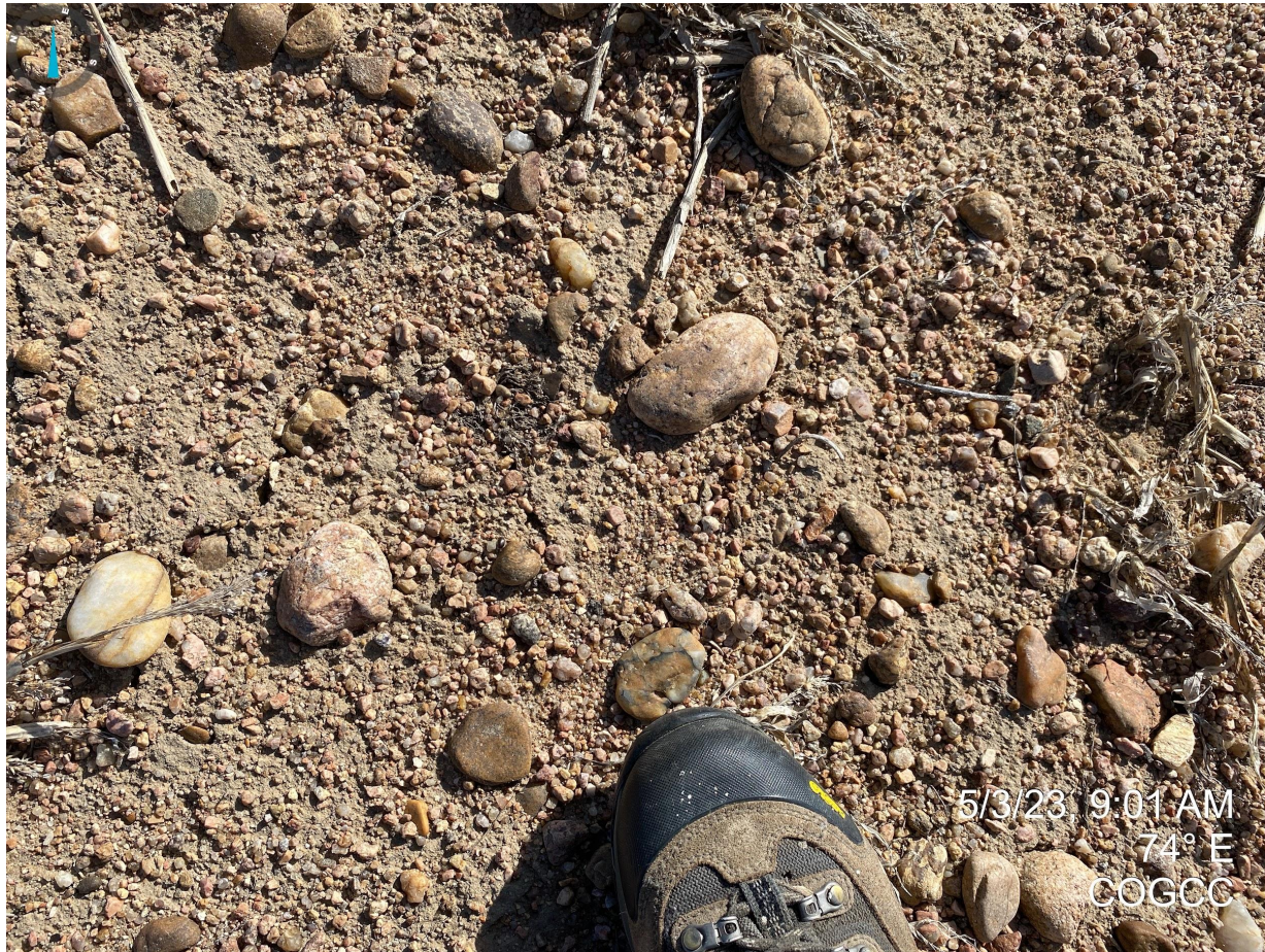
Photo 3. Close up photo of road base material left on the former production area and access road to well API# 075-05621.
