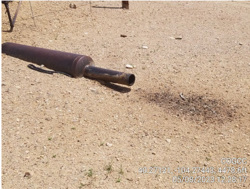
Photo 5 – Stained Soil at Exhaust
