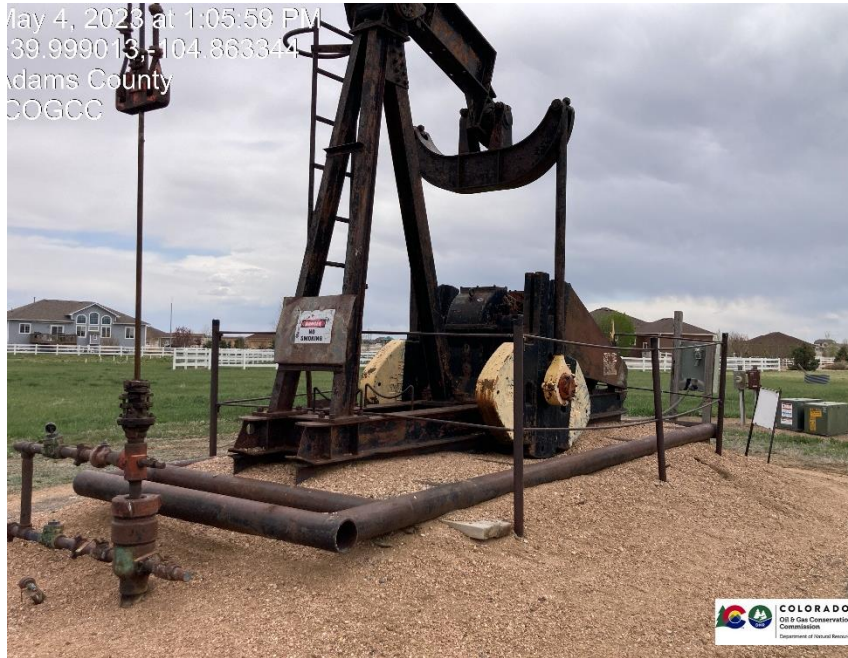
Pic 1 wellhead / pump jack
