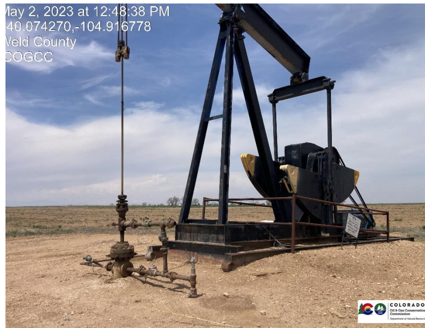
Pic 1 wellhead / pump jack
