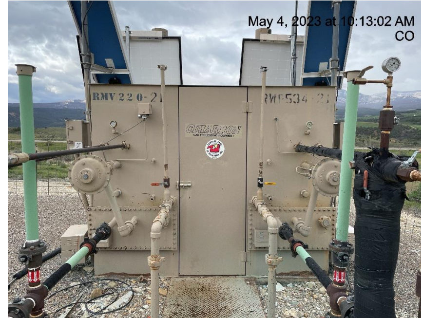
Photo # 6945 Meter calibration info not conspicuously posted
