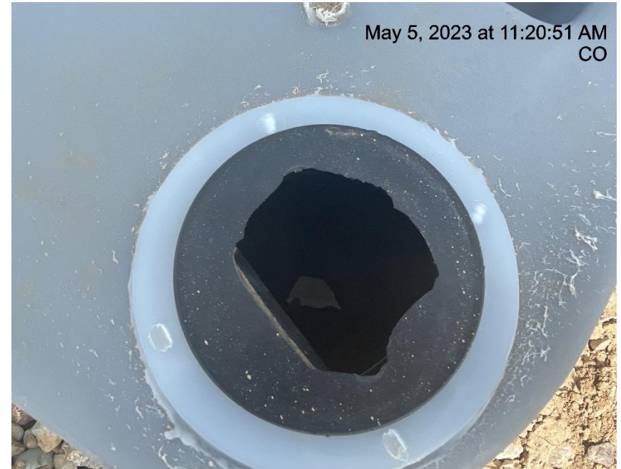
Photo # 7092 Chemical BMP 2/3 to 3/4 full of fluid/failure to maintain chemical BMP
