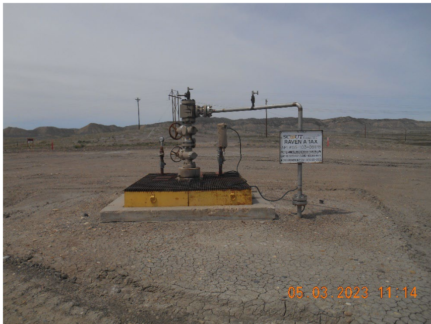
Injection wellhead
