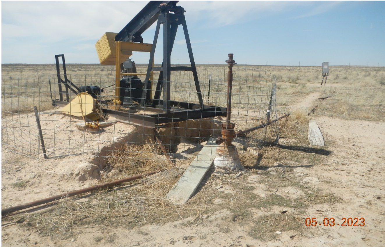
Photo 3. Facing toward the well head which appears inoperable. The base of the pumpjack has eroded and there are boards and debris around wellhead.
