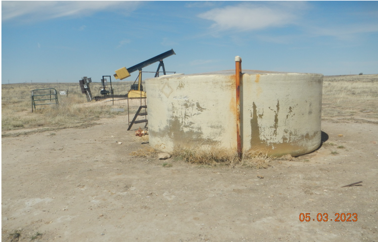
Photo 2. Facing toward the open top tank which still does not have secondary containment and does not have signage.
